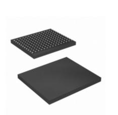
CYPRESS Part Number: CY7C1415KV18-250BZXC Manufacturer Cypress Semiconductor **Description** IC SRAM 36M PARALLEL 165FBGA Data sheet: CY7C14(11,13,15,26)KV18
